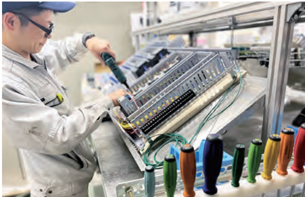
Dealing with manufacturing small-sized control panels
