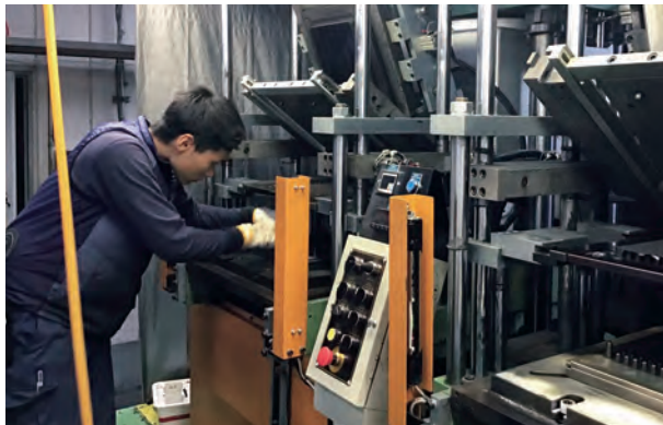
Greatly reduced defective products by vacuum forming machine
