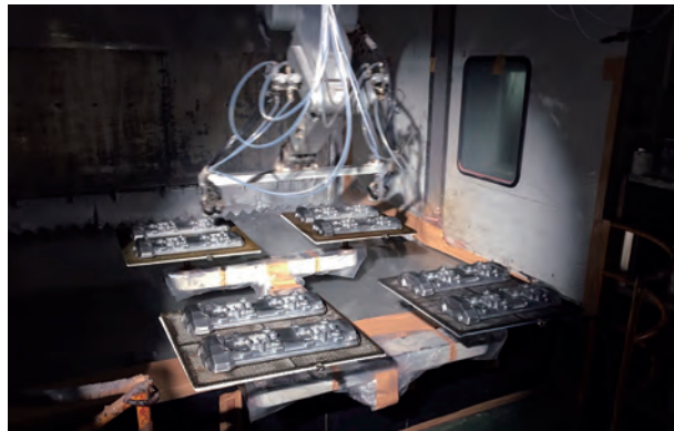
Operation painting robot in cleanroom of 100,000 cleanness level
