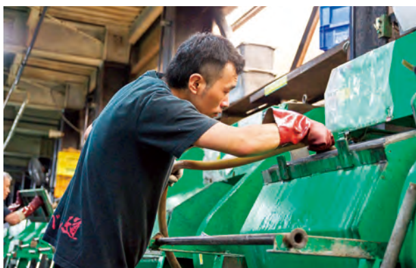
A fine adjustment of slewing polishing machine by pouring water
