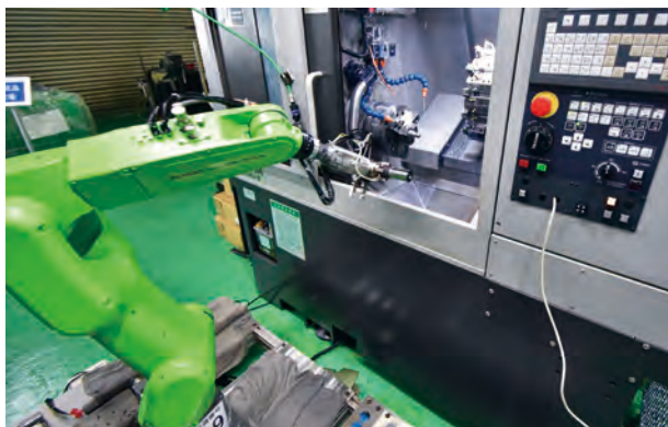
Removal work of products by robot.
