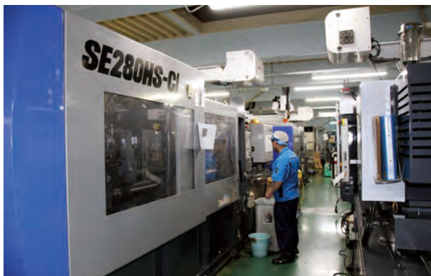
An electronic injection molding machine capable of processing dual-shot injection molding
