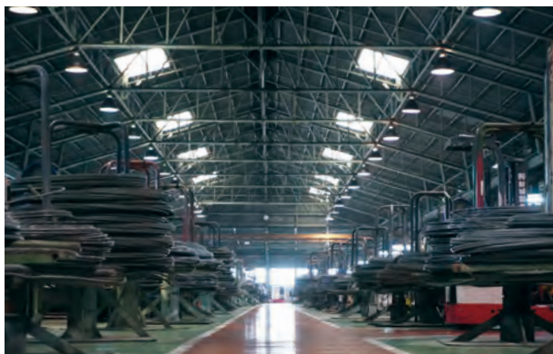
Forging machines that make five million nuts per day
