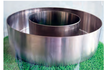
Large ultra-thin casing made from a turning center
