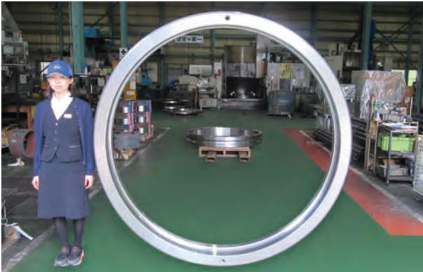
Bearing with an outer diameter of 2 meters made from a large-size turning center
