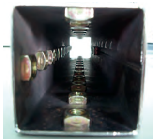
Pierce-clinch nuts installed in a square pipe
