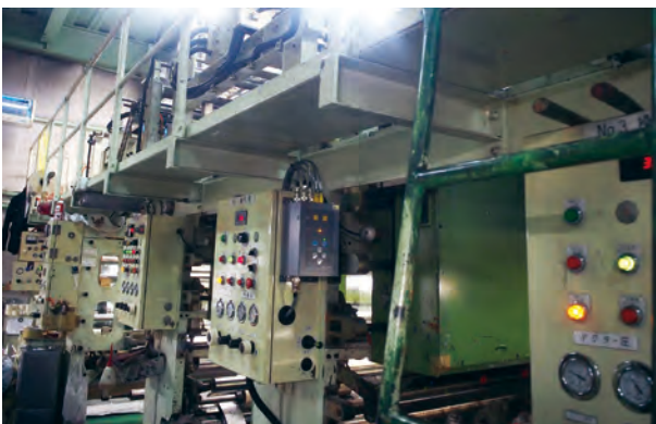
Rotogravure presses and automatic detection system at Tatsumi factory
