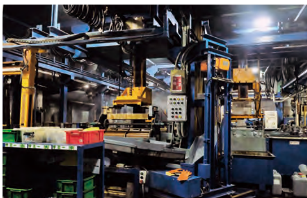
Facilities for sherardization process for screws and bolts
