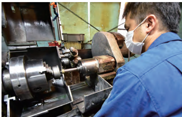
Picture of processing by internal grinder
