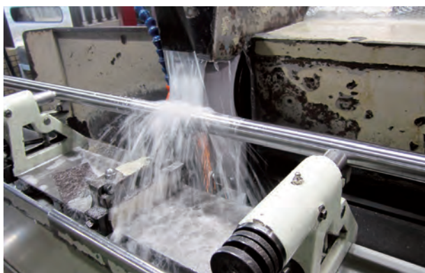
Polish thin and long object by using steady brace
