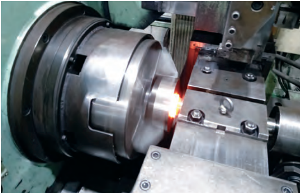
Condition of friction welding joint
