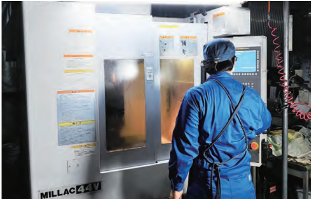
Cutting work by machining center
