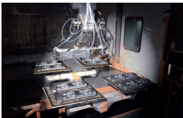
Operation painting robot in cleanroom of 100,000 cleanliness level
