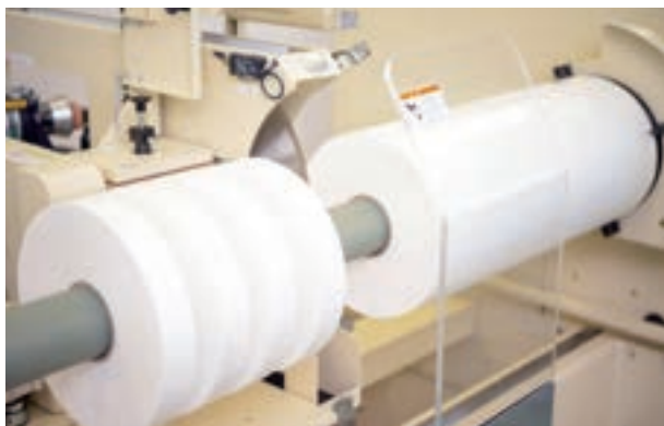
High speed full-automatic roll slitter
