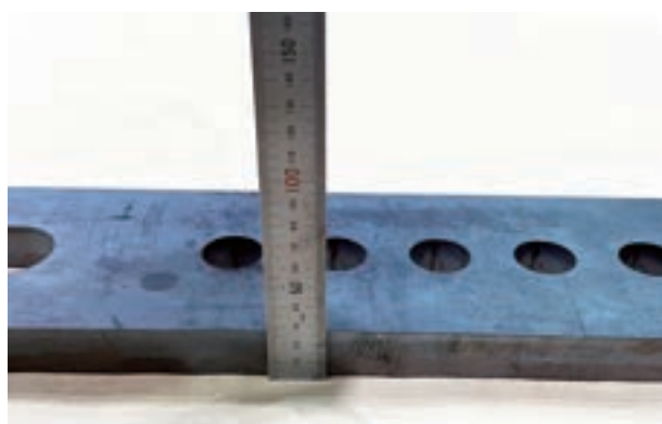
Heavy plate products by fiber laser processing machine
