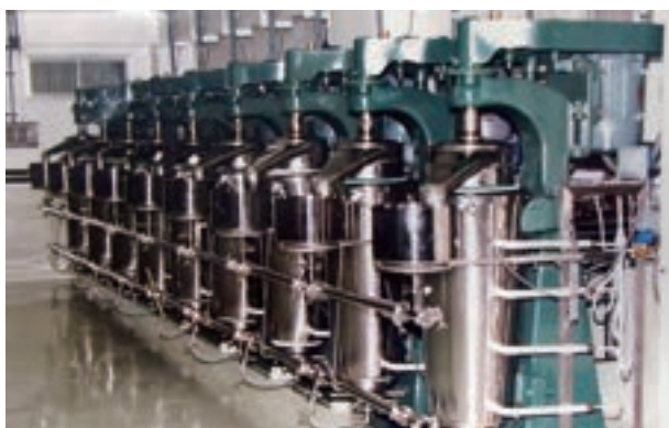
Centrifugal separator for producing blood derivative
