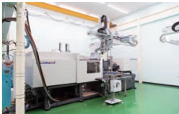
Manufacturing various plastic parts by injection molding machines
