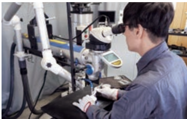
Laser welder at work under a microscope
