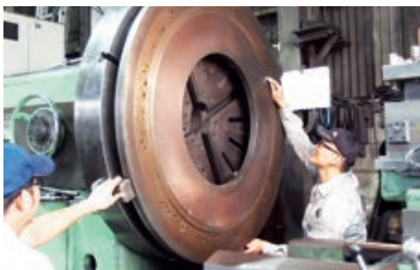
Front facing lathe with automatic tool feed mechanism for high difficulty machining
