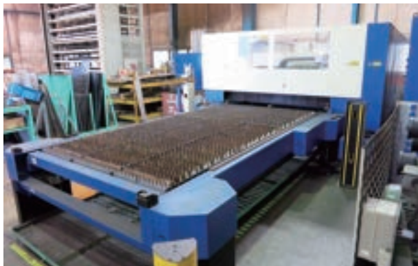
Laser cutting machines for precision cutting and small item cutting
