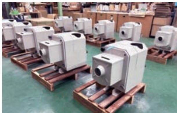
Enclosure of an oil smoke collector manufactured using advanced plate processing technology
