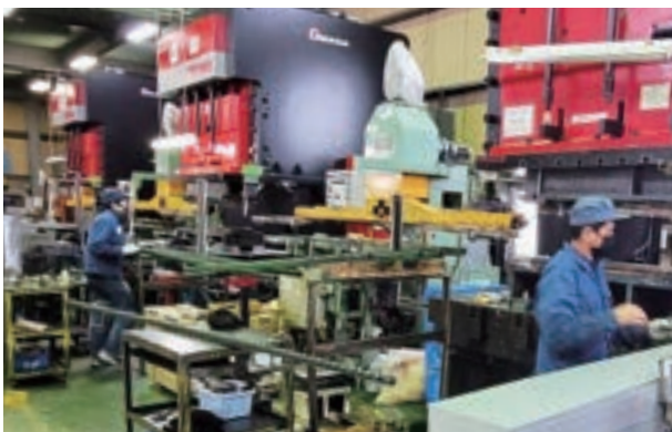
Manufacturing site with 250t presses
