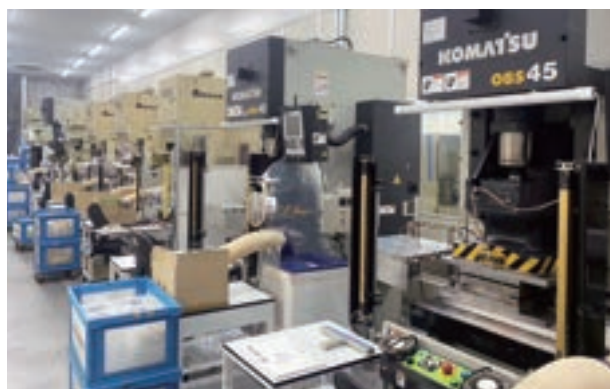
Forming process utilizing several presses
